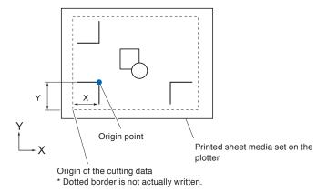
The origin point of the plotter will be set as the registration mark origin point as shown above, and it is different from the origin point of the cutting data. The difference between these two origin points are called as offset. In case of the figure above, set x and y to the cutting plotter as a registration mark offset.
