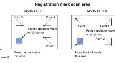
**3** Confirm the position of the tool, and if it is OK, press the [ENTER] key (SET).
